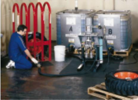
Over the last several years, OTR Wheel Engineering has become one of the premiere original equipment tire/wheel assembly providers in North America. Many of our original equipment customers require their tire/wheel assemblies to be flat proofed with polyurethane fills—also known as foam fill.
